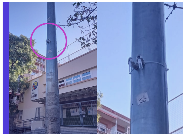
Figure 6 NO 2 diffusion tubes installed on lampposts
