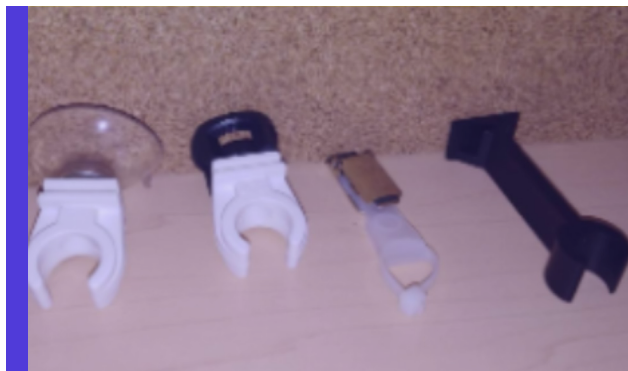
Figure 3. Types of NO 2 tube supports
