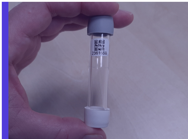
Figure 4. Palmes diffusion tube with the QR code attached (with both end caps)
