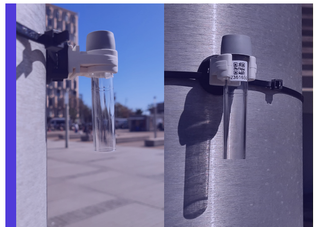
Figure 5 NO 2 diffusion tubes with a support
